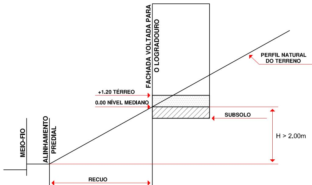
**TERRENO COM DESNÍVEL >2.00m EM DECLIVE**
